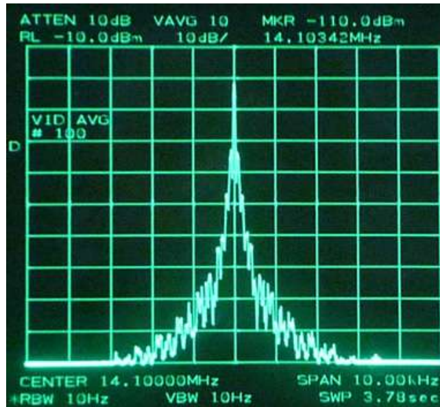
Fig. 21: Keying sidebands at \approx 50 wpm, 14.1 MHz, 100W.
