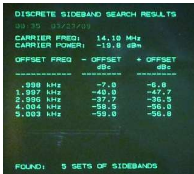
Fig. 17: AM carrier and sideband parameters.
