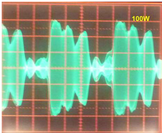
Fig. 14: 100W PEP speech envelope, 6 dB compression
